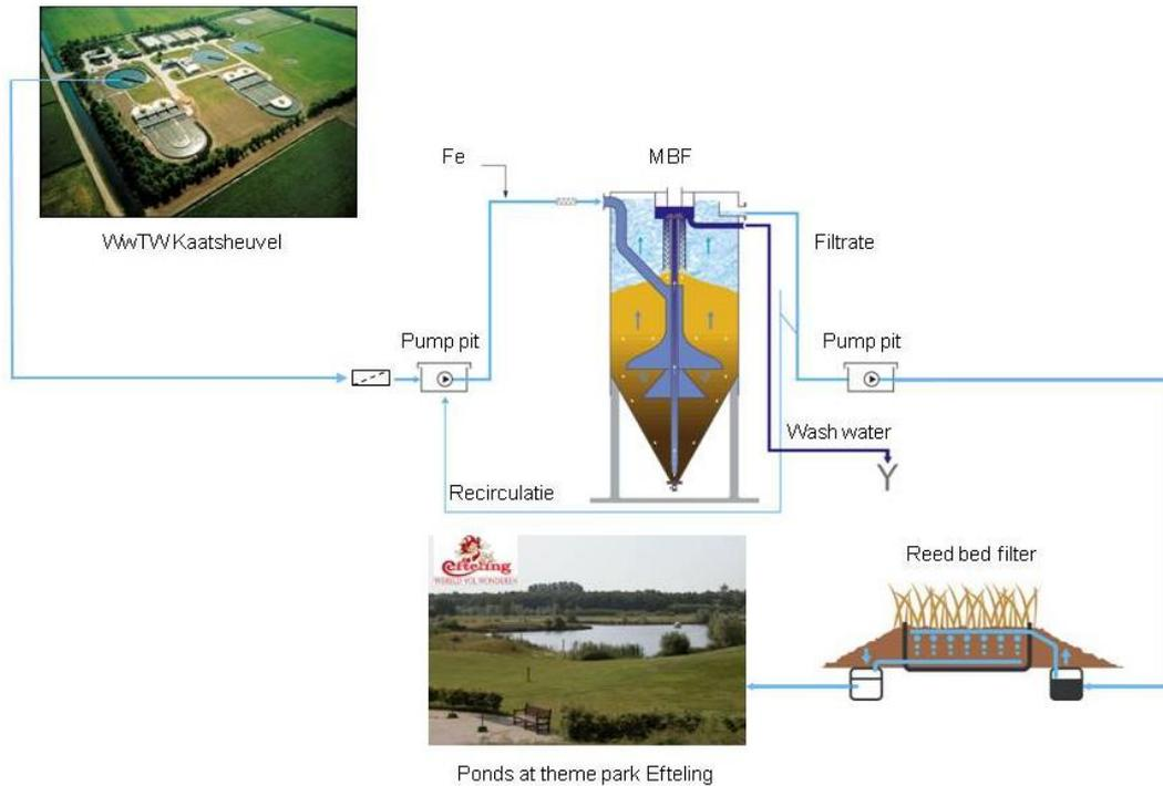
Figure 2 - Process scheme tertiary P removal treatment and reed bed filtration
