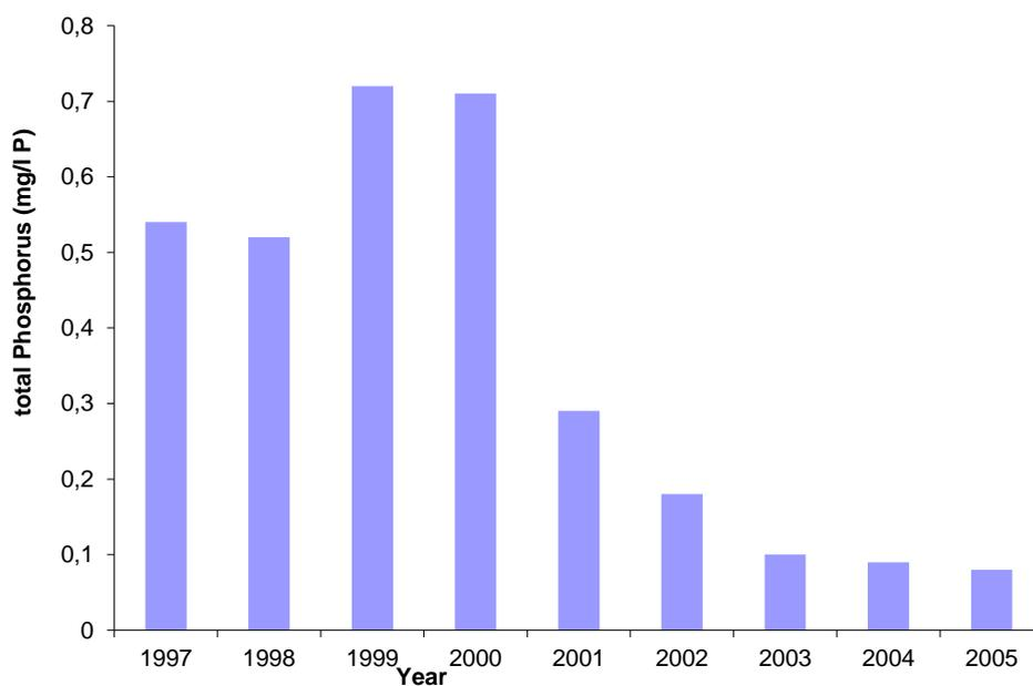
Figure 3 - Phosphorus removal at the tertiary filter plant of WwTW Kaatsheuvel
