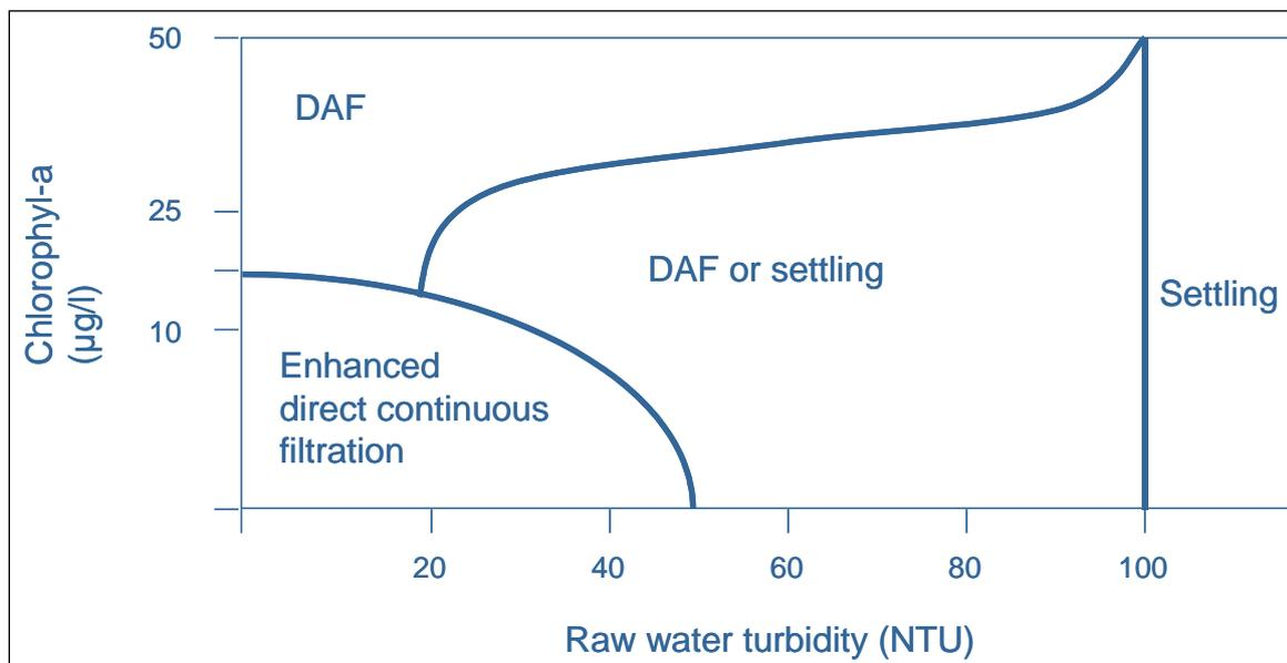
Figure 3: Surface water process selection diagram
