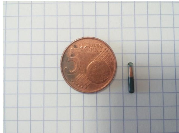
Figure 2 Illustration of the size of an RFID tag (right) on 0,5cm graph paper
